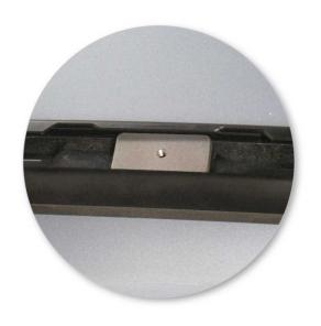
Slide metal T-nuts into tracks on vehicle. Two per track.
